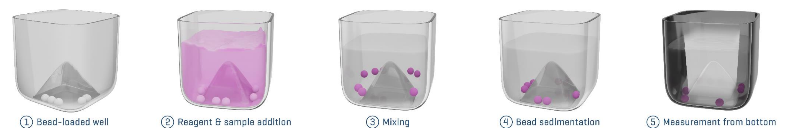
Figure 5. Workflow of the PA-201 glycan screening assay for Fc containing proteins. The whole assay is performed in the 384 well PAIAplates. Each well is pre-loaded with capture beads [1]. The lectin and the samples are added to the wells [2]. After shaking for 45 min [3] and bead settling [4], the plates can be measured on a fluorescence plate reader with bottom reading [5]. The whole process can be easily automated and takes roughly 60 minutes.
