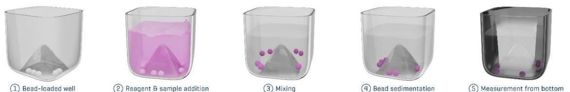
**Fig.2 :** Depiction of the workflow of the PA-201 assay in an exemplary well of the 384-well PAIAplate
