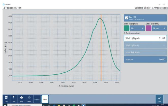
Figure 2: Screenshot of a Spark reader z-scan on a PAIA plate.
